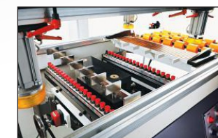
For vertical boring application. Both heads work parallel vertically
