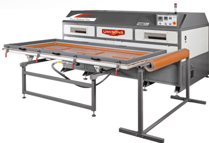
Work table with single side opening for easy loading
