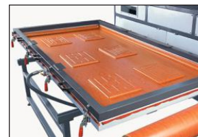
Work table with single side opening for easy loading
