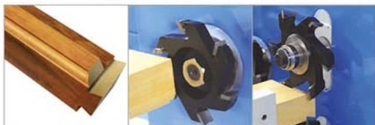
Cut The Dovetailed Male-end Of The Wooden Plank
