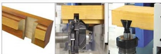
Cuts the matching female-slot of the wooden Plank
